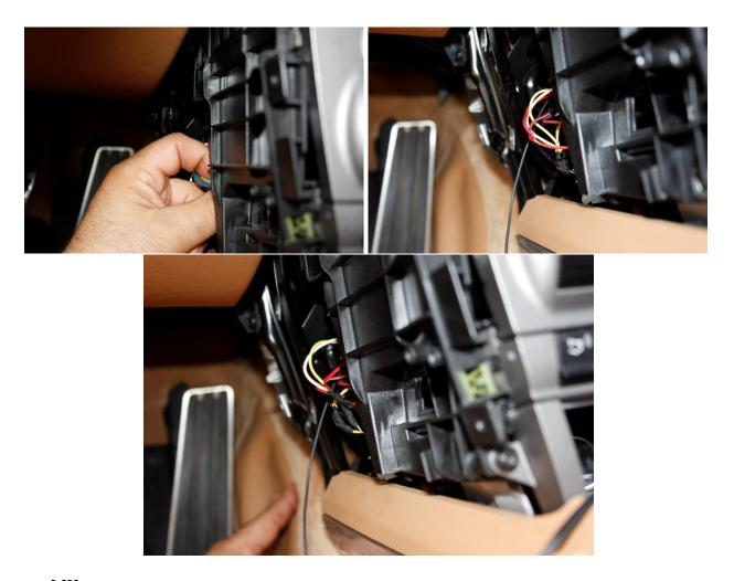
**VII.** Lastly, locate the large brown factory wire. Splice and solder to the black wire from the accelerometer. Once finished, wrap with electrical tape.
