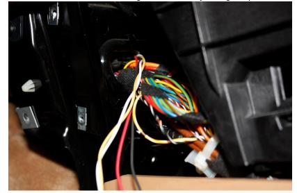
IV. Locate the main wire loom running through the middle console. Remove the wrapping, so that you can separate the wires. Locate the black/yellow pair of wires (both with white tracer) and untwist.
