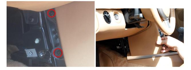
**II.** Attach the provided wire harness to the DSC accelerometer. Ensure that locking tabs are engaged and all corresponding wire colors line up accordingly. Using the 3M adhesive provided, attach the accelerometer atop the factory 2-axis accelerometer located in the middle console, to the right of the accelerator pedal. Ensure that wires are facing the front the car. The accelerometer will fit snug between the 2 parts as shown below.
