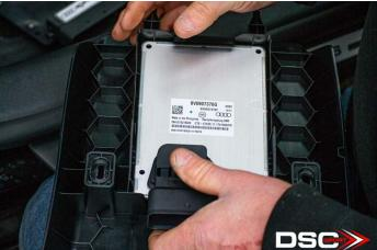
11. Disconnect the factory controller from the harness by pulling the slide lock gently and then pull the module away from harness
