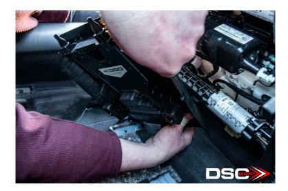
5. If purchased, now is a good time to run a USB cable to the top of the controller, and out under the edge of the cover
