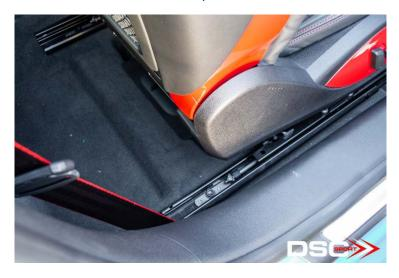
5. Remove the remaining two m10 triple square bolts
