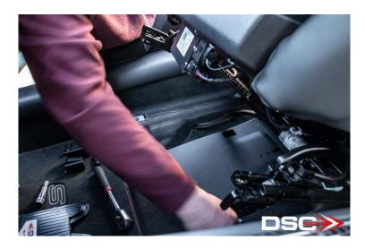
8. To remove this panel there is a 10mm nut on each holding the cover down. Remove both of these nuts.
