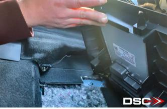
10. Now pull out the factory module from the cover by spreading the retainer bracket away from the controller
