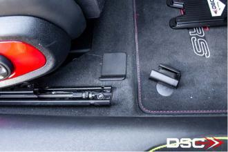
3. Once end covers are removed, use a m10 triple square to remove the seat bracket bolts
