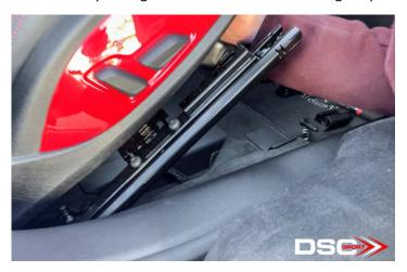
4. Move the seat position all the way forward and reinstall the m10 triple square bolt on the rear of each seat rail
