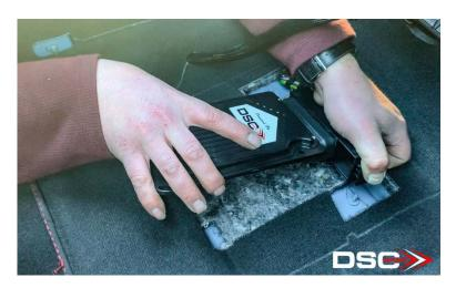
4. Install the new DSC controller into the factory bracket. Begin by place one side in the bracket and then while pulling back the other side, the controller should snap right in. Then slide the controller up to the top clip.
