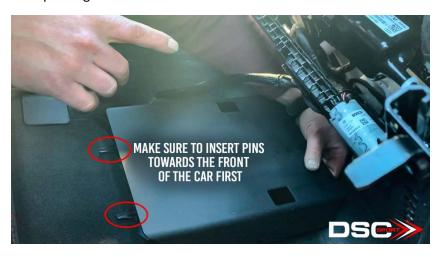
2. Reinstall both of the 10mm bolts on the top of the cover
