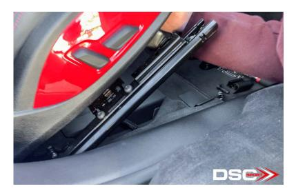
7. This will now reveal a plastic cover under the seat. This is where the factory control module is located.
