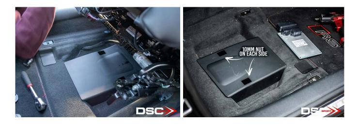
9. Remove the cover by pushing it towards the rear of the vehicle while also lifting up
