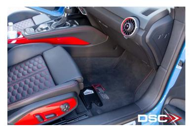
2. Find and remove front plastic end covers on each side of the seat rail
