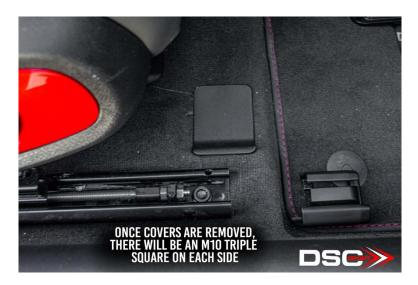
4. Next slide the seat all the way forward to reveal two more m10 triple square bolts at the rear of the seat rails
