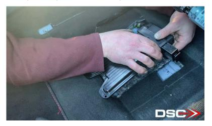
3. Once the connector is around the DSC controller, begin to push the locking slide clip inwards and it will pull the controller the rest of the way in. Check to make sure the controller is fully locked in and will not slide out.
