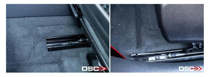
5. Move the seat all the back towards the rear of the car and reinstall the m10 triple square bolts on the front of each seat rail
