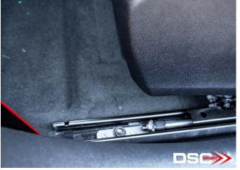
6. Once all four seat rail bolts are removed. Return the seat back to the centered position and then tilt the seat back towards the rear seat of the car
