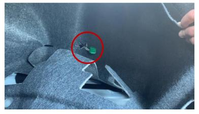
7. Install the two screws back on the rear trim panel
