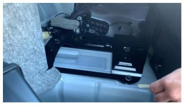
4. Tighten down the five 13mm bolts for the subwoofer and controller bracket (only reinstall the two bolts on the controller bracket if no subwoofer is equipped)
