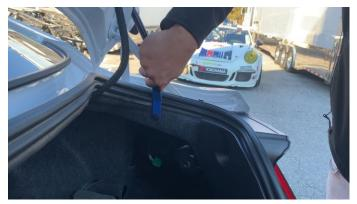
8. Pull back the carpet revealing the suspension control module
