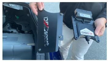
2. Attach controller to bracket by placing the backing plate and allen head bolts on the back of the controller through to the bracket
