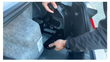
11. If the car does not have the factory subwoofer, it will only have three 13mm bolts on the module bracket
