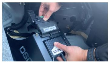
7. Once aligned, begin to close the lever on the connector. This will draw the two together. There is no need to push
