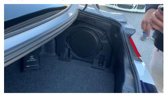
2. Remove the cargo area carpet panel by simply lifting and pulling it towards you.
