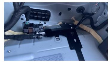
12. Pull the entire module assembly towards you to gain access to the harness
