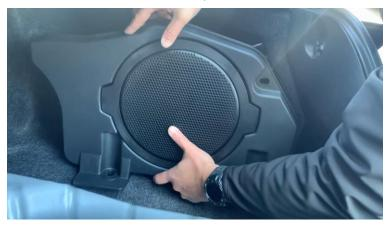
9. Tighten down the three 13mm bolts on the front of the subwoofer
