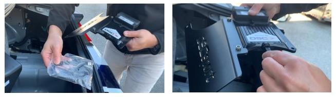
5. When installing the DSC controller back into the car be sure to have the harness running towards the outside of the vehicle
