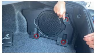
4. Slide the subwoofer slightly and disconnect the green connector behind it
