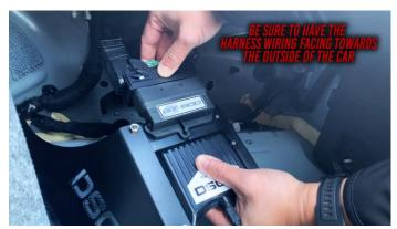
6. Gently place the connector back onto the DSC controller, making sure not to force it (this could result in bent pins)
