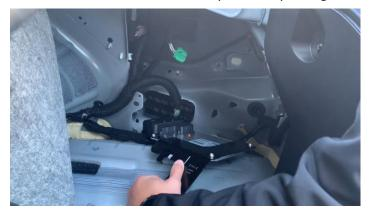
13. Pinch the tabs on each side of the harness to release it and begin to pull up slowly
