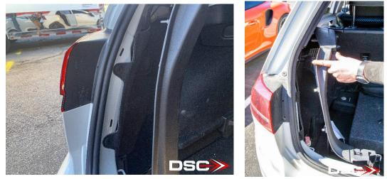
9. Remove the 2 push pins holding the carpet on. Use of a pry tool will help here.
