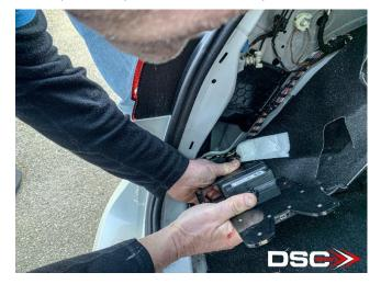
3. Once the connector is around the DSC controller, begin to push the locking slide clip inwards and it will pull the controller the rest of the way in.
