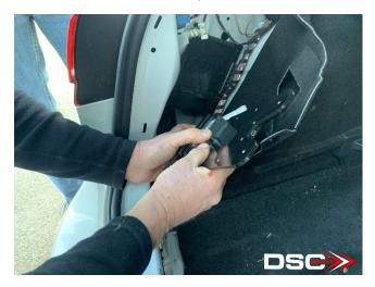
4. Check to make sure the controller is fully locked in and will not slide out.
