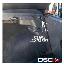
8. Pull back the side trim panel by running your fingers along the panel starting from the where the trunk latch trim panel was just removed. You do not have to remove the panel fully, just enough to get to the wheel well area.
