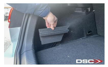
2. Remove the cargo area carpet panel by simply lifting and pulling it towards you.
