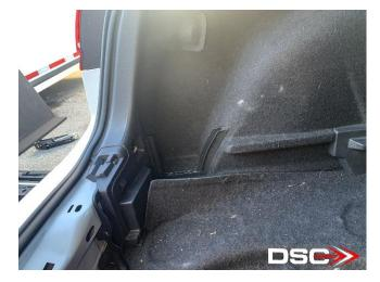
4. Clip back in the trunk latch trim panel. Begin by lining up the 6 plastic hooks inside of the trunk. Once lined up press down on the top to insert the 4 clips along the edge.
