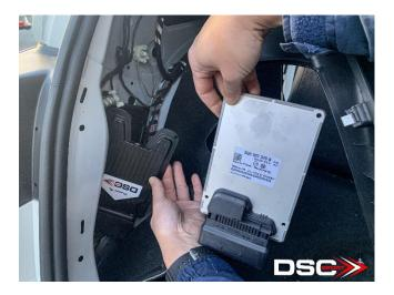
5. Install the new DSC controller into the factory bracket. Begin by place one side in the bracket and then while pulling back the other side, the controller should snap right in. Then slide the controller up to the top clip.
