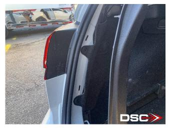
2. Clip in the driver side upper panel. Be mindful of the white pin on the backside that will need to be lined up with the hole in the body of the car. Once in line up the 2 side clips on the trunk opening and push in. And snap in the lower plastic near where the T30 screw originally was.
