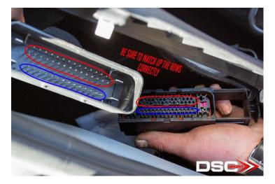
2. Line up the connector and begin to gently seat the controller into the harness. You do not need to force it in. If lined up correctly, it will slide on easily.
