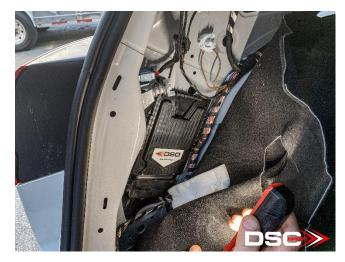
6. If purchased, now is a good time to run a USB cable to the top of the controller, and through the hole in the carpet right behind the wheel well.
