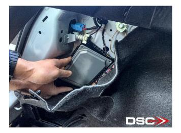
12. Disconnect the factory connector by pulling the slide lock gently.
