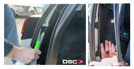
10. Pull back the carpet revealing the factory control module.
