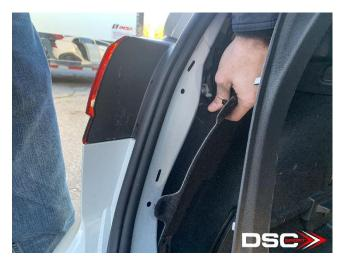
11. Remove the factory unit from the bracket by slightly prying out one side with a flat head screwdriver.
