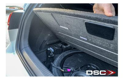
3. Disconnect the subwoofer connector and remover the subwoofer enclosure.
