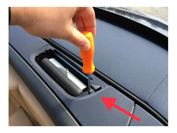
4. Remove the large trim panel by gently lifting the panel upward one side at a time.
