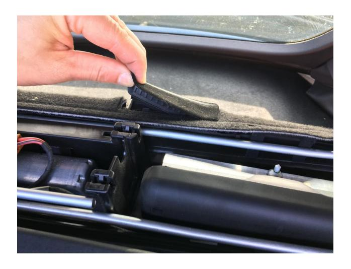
7. Release the "hooks" that hold the rear carpet. There is a total of 3 hooks(one in the middle, and one at each end).
