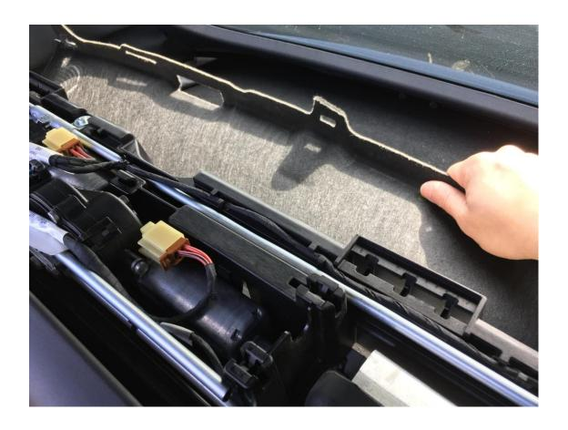
8a. With the carpet pushed back the OEM PASM controller will be exposed (it is the silver color box). The controller is seated on molded foam tray. There's nothing else holding it in place.
