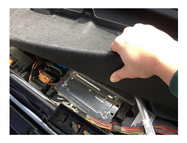
9. Lifting the controller up from the molded foam tray and then carefully remove the two slide-lock connectors(see 9a).
