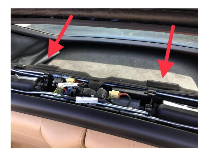
6a. The rubber inserts will come off by lifting upward.
