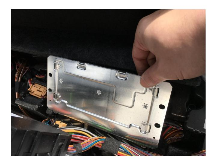
9a. Unlock one slide-lock connector at a time by gripping the connector and sliding it to the direction of the arrow in the image. Again, unlock only one connector at a time. Once the two slide-lock connectors are released the controller can then be removed from the car.
