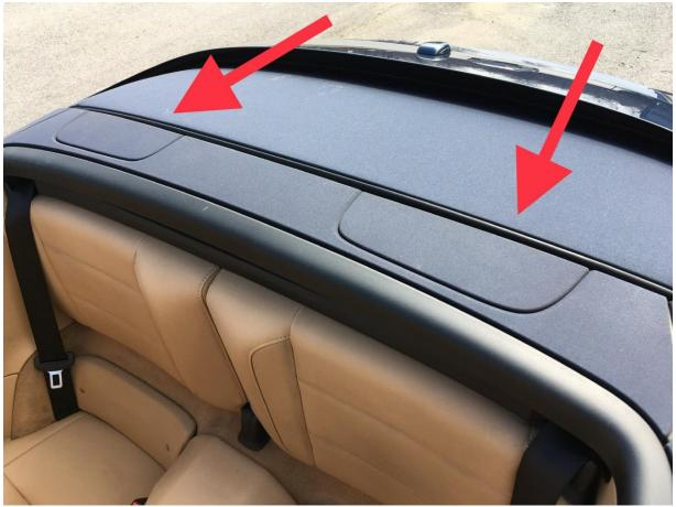
2. Carefully remove the two small trim panel by lifting by the rear edge. A plastic wedge tool may be used to "pop" up the rear edge. I found that using only my fingers worked fine.
