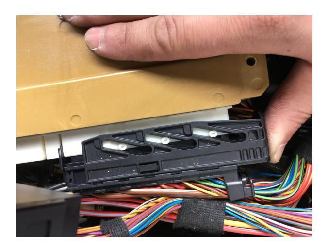
10a. Make sure the slide-lock connectors are fully engaged shown in this image by the pegs in the diagonally slots.
