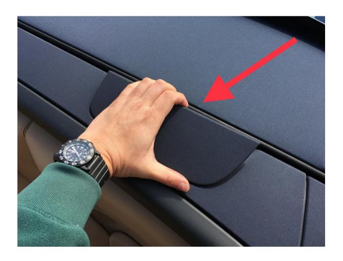
3. Remove the Phillips screw on each side of the trim panel. There's 2 screws(one on each side).
