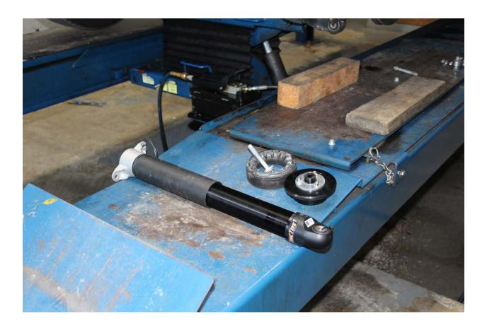
3. The DSC Sport rear adjustable spring perch is to be installed in the control arm on the bottom of the divorced spring location, this will have to be disassembled to install. Remove the three socket head bolts to install like shown.
