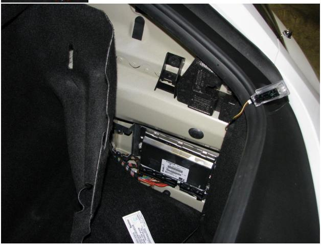
Without disconnecting the battery, replace the OEM Suspension controller with the DSC Sport controller. It is a direct replacement so remove the OEM controller then remove the connectors, reconnect to the DSC Sport controller then mount in OEM location.
