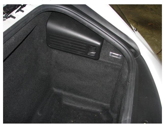
Pull back on the cover and carpeting to expose the OEM Suspension Controller.
