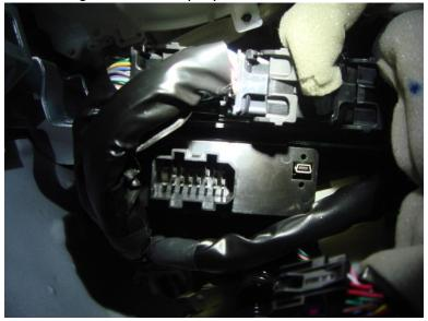
**VII.** Connect wire loom to DSC Sport controller's connector.
