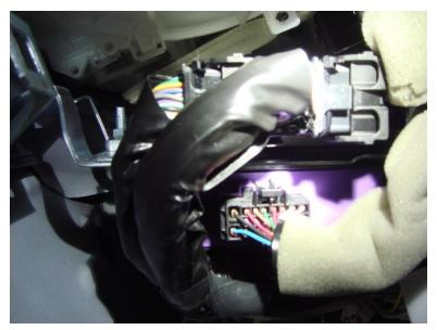
**V.** Carefully remove the connector and board from the controller's cabinet (move side to side as you pull the board out). Once the board is removed from the cabinet, disconnect the wiring loom.
