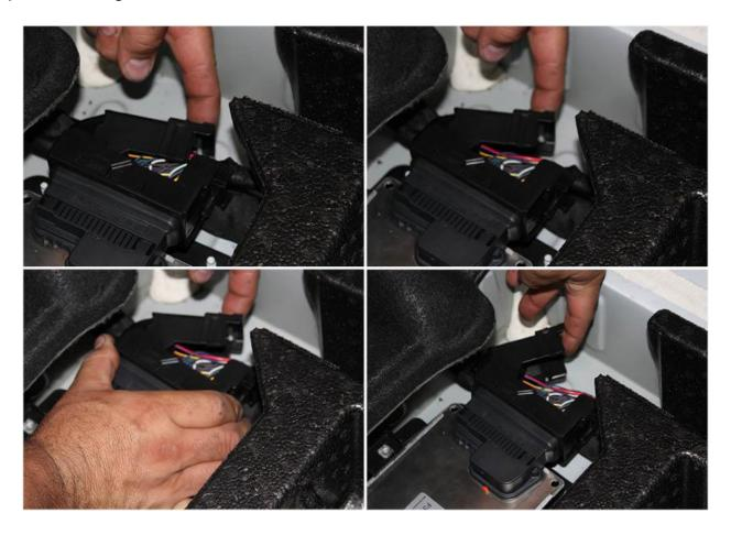
**4.)** Once unlocked, remove controller from connector.
