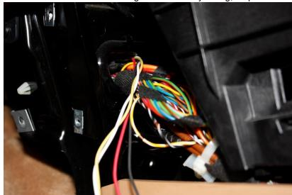
Locate the main wire loom running through the middle console. Remove the wrapping, so that you can separate the wires. Locate the black/yellow pair of wires (both with white tracer) and untwist.
