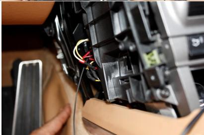
**VII.** Lastly, locate the large brown factory wire. Splice and solder to the black wire from the accelerometer. Once finished, wrap with electrical tape.
