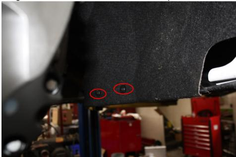
**VII.** Using a flathead screwdriver, remove the two plastic snap rivet fasteners pictured below.
